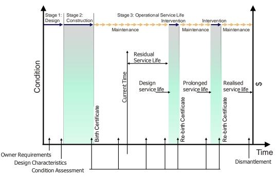
Fig. 1 – Phase in the life of a structure from Model Code 2010
